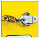
Attach anchor plate (D) and pre-assembled chain / fusible link assembly (A) onto the side of the cabinet using self-tapping, metal screws (B). The straight length of the D-ring attached to the fusible link assembly should sit and rotate freely under the raised portion of the anchor plate.
