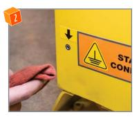
Ensure the connection area between the grounding wire and connection point is clean, secure, dry, and free of rust and paint.
