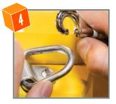
While holding the door open, insert the spring clip into the door mounted D-ring to hold doors open. Operate spring clip as necessary to hold door open.
