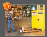
Remove additional safety support materials and lower the cabinet slowly onto the floor.
