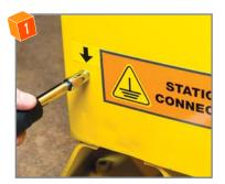
Remove the grounding screw from the cabinet with a nut driver or socket.
