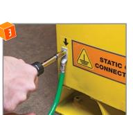
Place grounding wire connection point securely around the grounding fastener and tighten into slot on cabinet wall.
