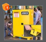
Using a bubble level, access each leveling foot through the top of the bolster and adjust with a 1/4" socket or nut driver until the cabinet is fully level [front / back and left / right]
