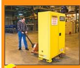
Place a forklift or pallet jack squarely underneath the cabinet and lift approximately 4-5".
